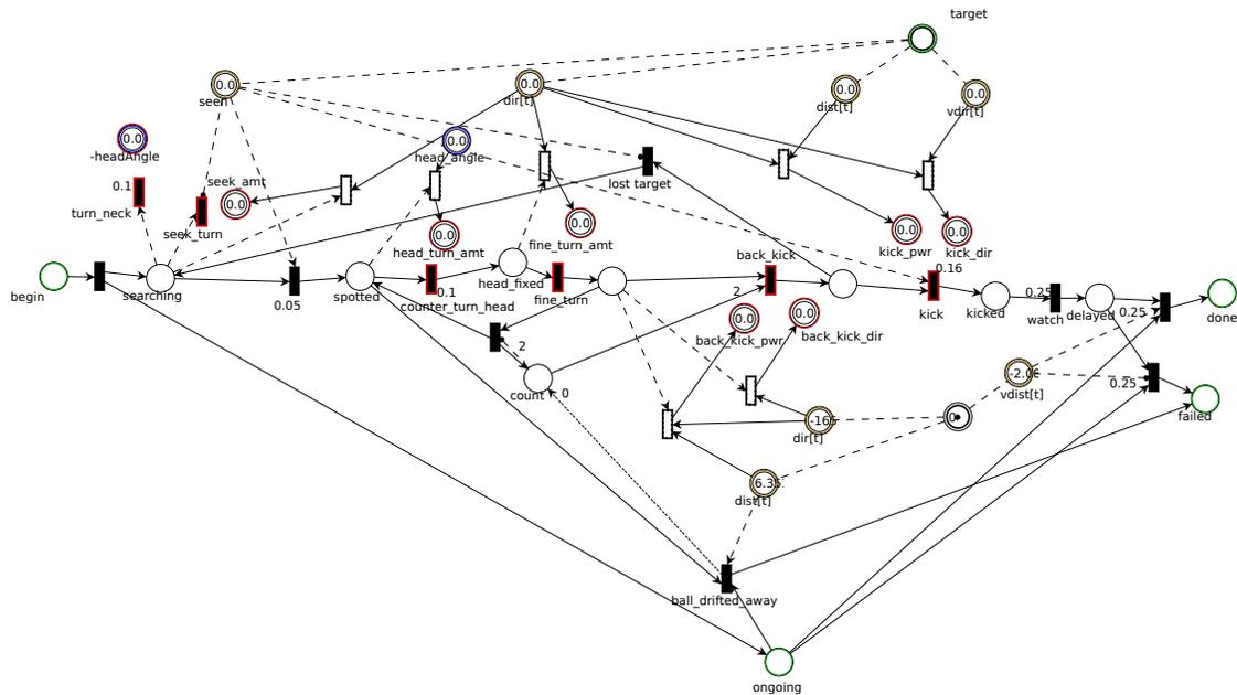
Figure 4.4: The low-level behavior to *pass* the ball to a teammate. If the distance to the ball grows too high while it orients toward the teammate, it recognizes this and goes to the *failed* state.
