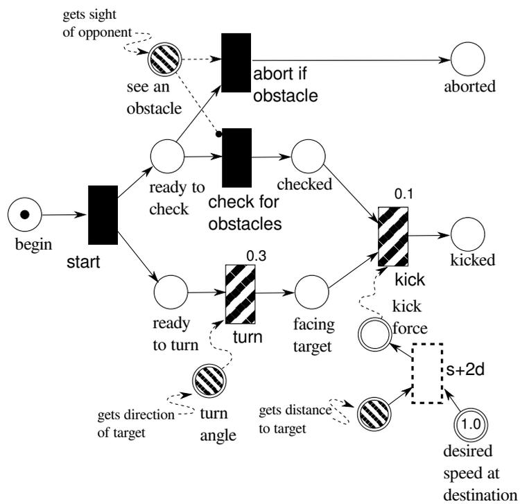
Figure 2.9: Here, we show how the kick network uses continuous inputs to make decisions and set its control outputs.
