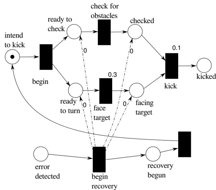
Figure 4.1: Here, set arcs from the *begin recovery* transition put the entire module into the desired state.
