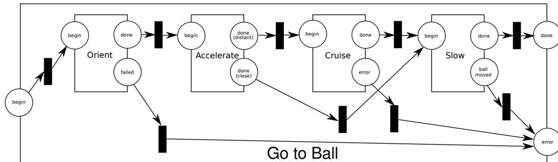
Figure 3.1: A behavior to approach a stationary ball.
