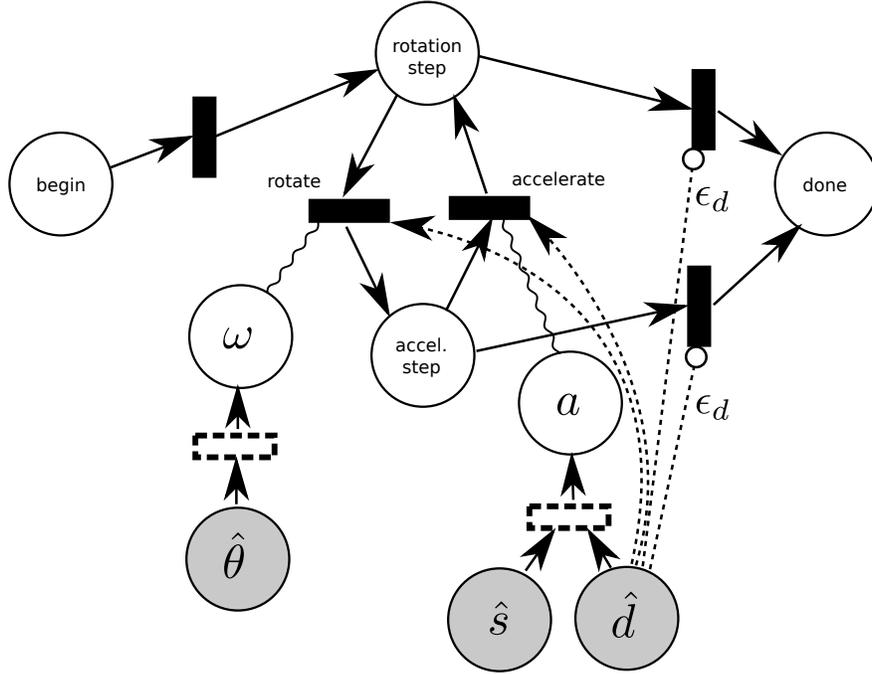
$$\begin{aligned} \omega_{t+1} &= -\hat{\theta}_t \\ a_{t+1} &= \frac{1-\gamma}{(1+\delta_s)(1+\delta_a)} \left( \frac{1}{1+\hat{\delta}_d} \hat{d}_t - \frac{1}{1-\hat{\delta}_s} \frac{\gamma}{1-\gamma} (1+\delta_s) \hat{s}_t \right) \end{aligned}$$
