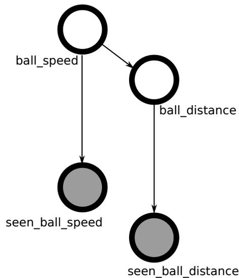
Figure 2.16: In standard Bayes net notation, observed variables are shown as shaded. Here, the soccer agent observes the variables *seen\_ball\_speed* and *seen\_ball\_distance*; based on this information, it can infer the distributions of the other variables.
