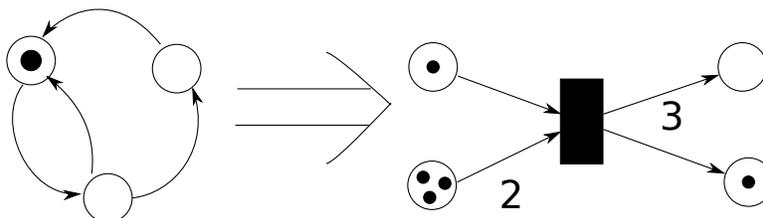
Figure 2.2: Finite state machine compared to Petri net
